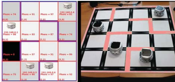
Figure 7: Robotic implementation of the EVAP algorithm on the tiles emulator
